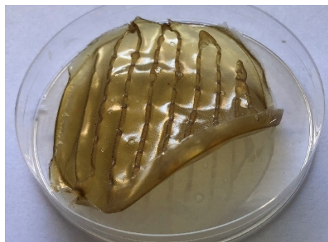
Figure 3: Three-dimensional shape of chitosan layer – the bend is aligned with the lines being dispensed on the layer.
