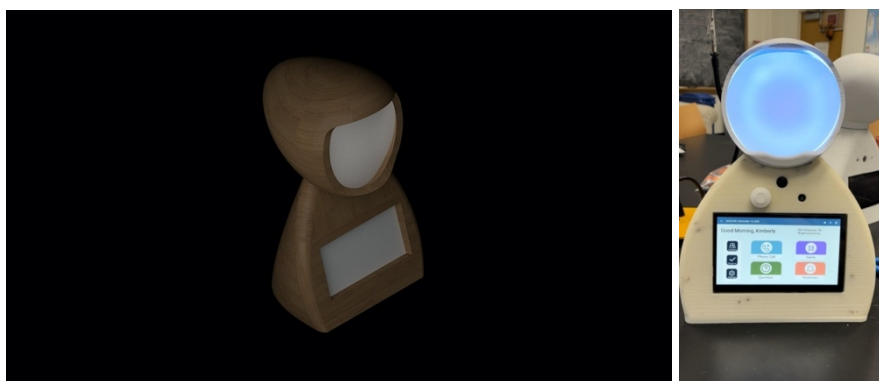
Figure 1: Body design concept and finished prototype. The prototype features a wider body to accommodate the larger screen, and a more relaxed face visor to make the appearance more friendly.
