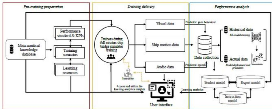
**Figure 3:** Overview of performance evaluation system in nautical simulations.
