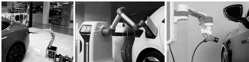
Figure 4: Selection of prototype systems for conductive side coupling. Left: Tesla charging snake (Tesla, 2016); middle: VW charging robot (Volkswagen AG, 2022); right: Kuka Carla connect (Kuka AG, 2021).
