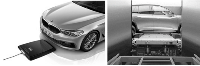
Figure 1: Examples of inductive charging (BMW wireless charging, 2022), left, and battery swapping (Nio, 2022), right.
