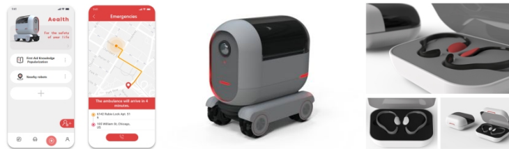
Figure 7: Product effects, (A) mobile interface design; (B) AED first aid robot; (C) wearable heart rate detection device.
