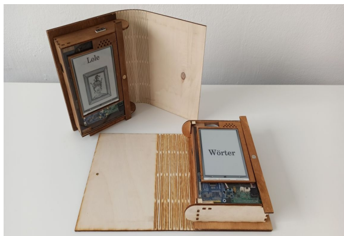
Figure 1: Left-hand and right-hand version 1 prototypes of Personal Primer (PP) artifact with integrated speech capabilities, e-ink displays, circadian module (Hromada, 2021), solar panel and touchless gesture command & control interface.
