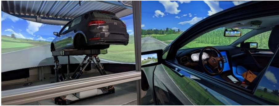
Figure 3: (a) The dynamic driving simulator used in the study; (b) image of the interior of the car. The larger touchscreen display in the centre was used for the graphical user interface.
