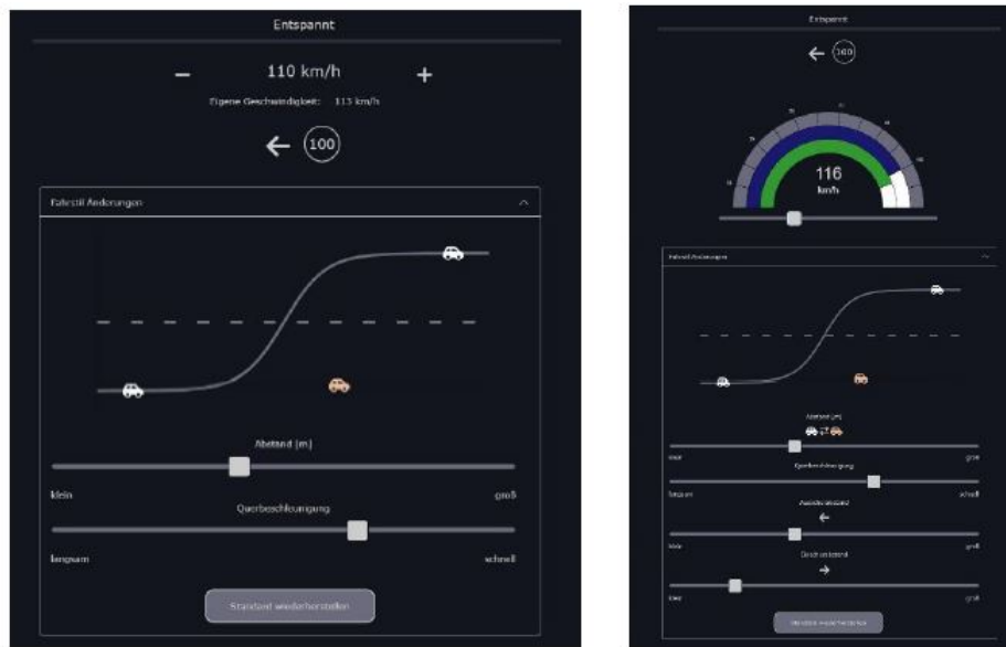
Figure 2: (a) The basic HMI allows the users to adjust the THW and lateral acceleration during an overtaking manoeuvre; (b) the complex HMI also gives the users the possibility to change the THW for initiating the overtaking manoeuvre and the distance for initiating a lane-change to complete the overtaking manoeuvre. Furthermore, it shows a more complex speed display and allows the users to change the desired speed with a slider.
