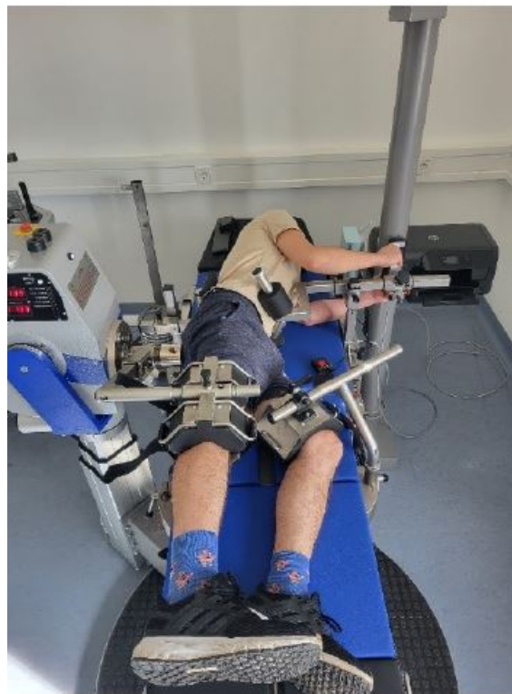
Figure 1: Positioning of the subject for the isokinetic and isometric force measurements.
