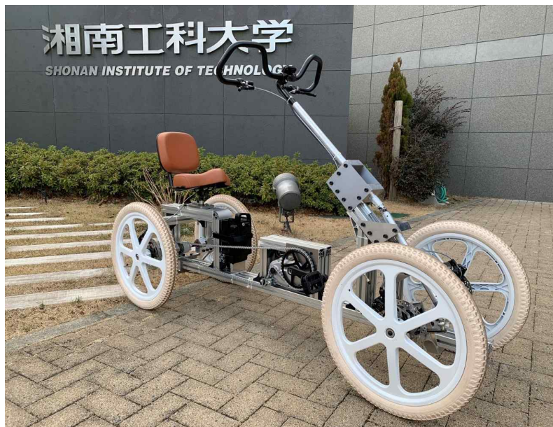
Figure 8: Prototype of the underpart of Quadricycle for their 20s to 30s women day-tripper to the Shonan area (SQC-01).
