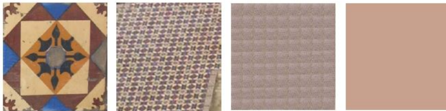
Figure 4: Changes in perceived colour, depending on the observation distance (source Gamito, 2013).
