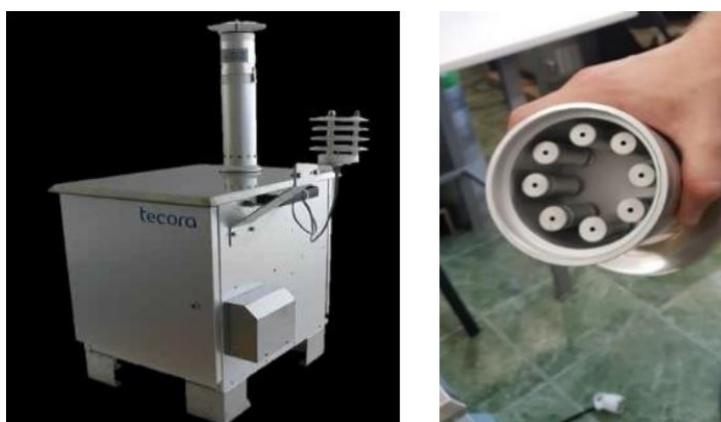
**Figure 1:** TECORA SKYPOST PM-HV sampling device.
