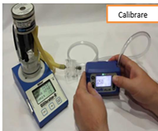
**Figure 2:** GILAIR PLUS air sampling device.
