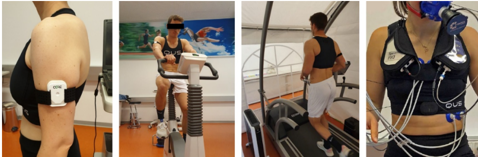
Figure 1: Setup for sensor evaluation in standardised and heat conditions. Gold standard reference sensors with 6-lead ECG and spirometry (rightmost).
