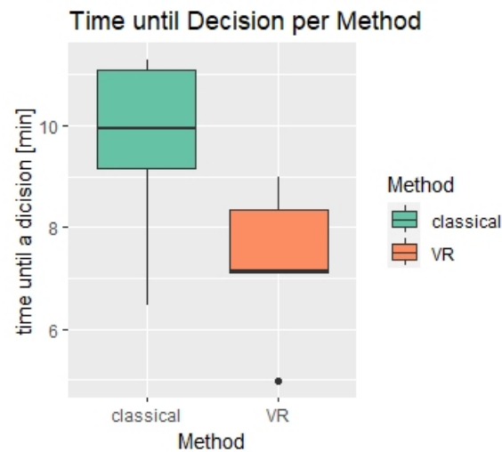
Figure 8: Time needed until a decision about a cable length was made in both VR and the classical method. The horizontal line represents the median.
