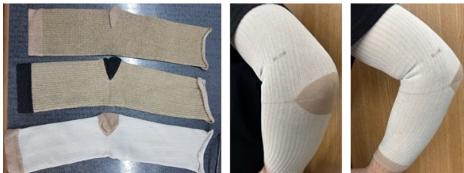
Figure 2: Tubular conductive textile structure.
