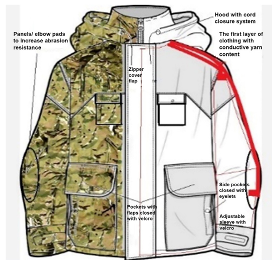
Figure 1: Jacket with the first layer having conductive yarns.
