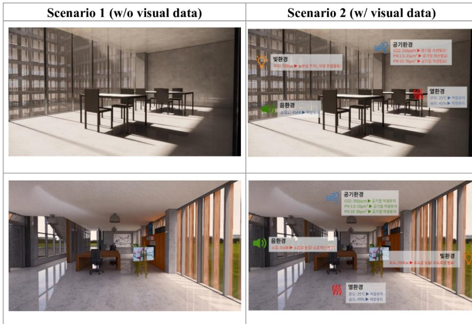
Figure 2: Example of IEQ visual data in pictograms in a 3D virtual space.
