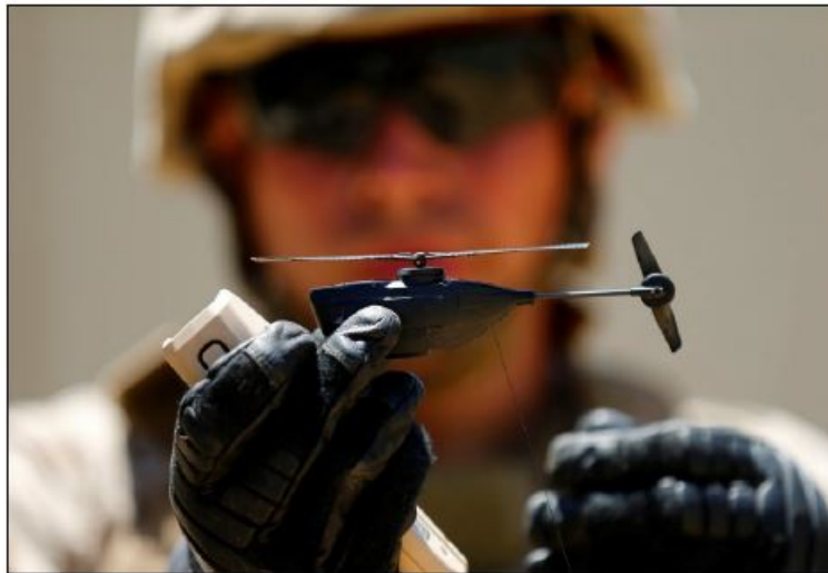
Figure 1: Small drones like the Teledyne/FLIR Black Hornet can get close to a person or area of interest without being seen or heard but are particularly challenging to control and highly susceptible to environmental conditions (e.g., wind).
