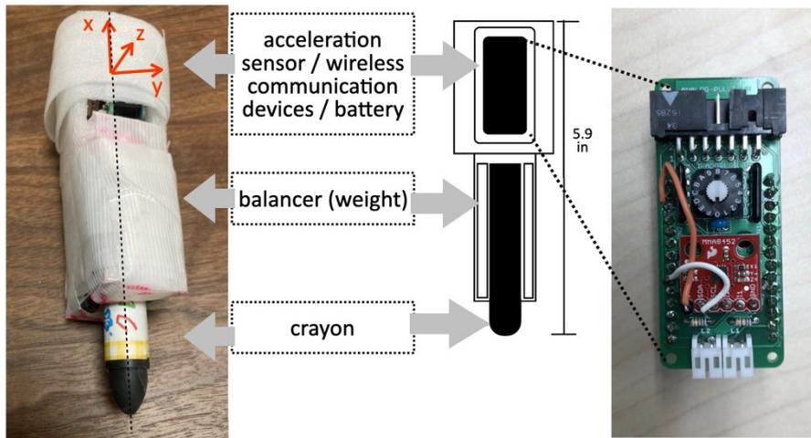
Figure 2: Prototype of pen-holder type device.
