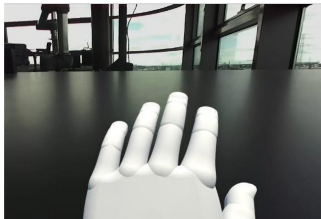
Figure 5: Augmentation of the haptic glove in the live visual feedback from the camera.
