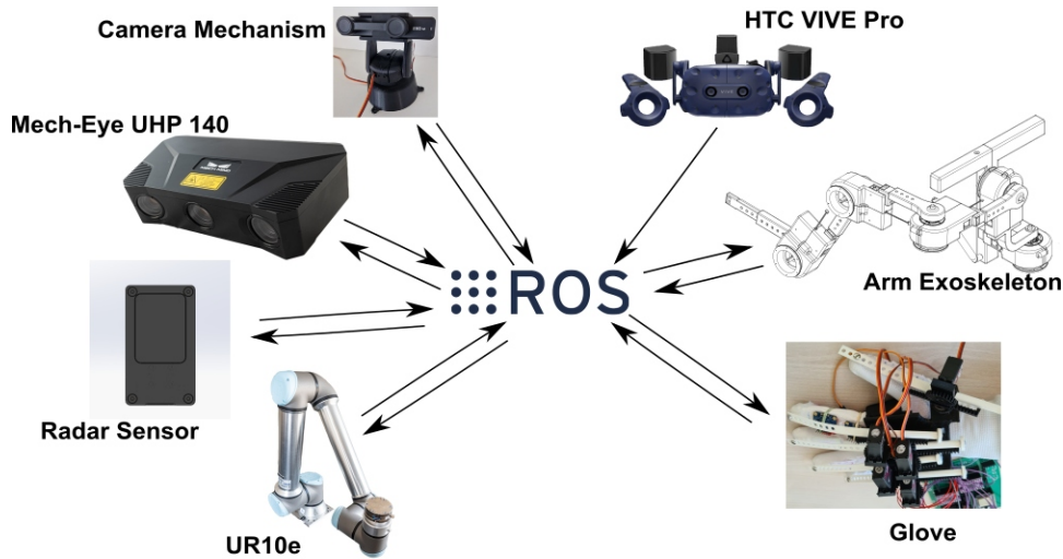
Figure 4: Architecture of the signal interface environment.
