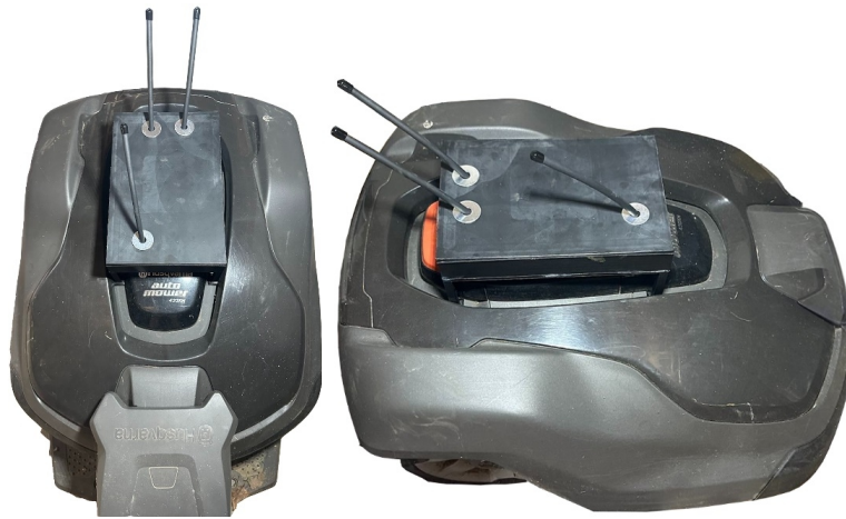
Figure 4: SATCRUISER payload mounted to the automower UGV in the charging dock (left) and out of the dock (right).
