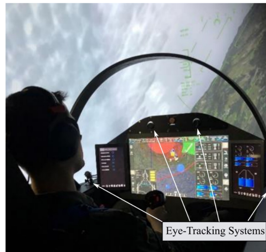
Figure 1: A Pilot operating UAVs interacts with the cockpit interface during an experiment. The touch-sensitive tactical map is used to task the UAVs. Each gaze interaction is tracked and passed by the eye-tracking system. Then, the observation generation in the aircraft interface uses the semantics of each gazed instrument to infer what information the pilot perceived at a given time, according to (Mund and Schulte, 2017).
