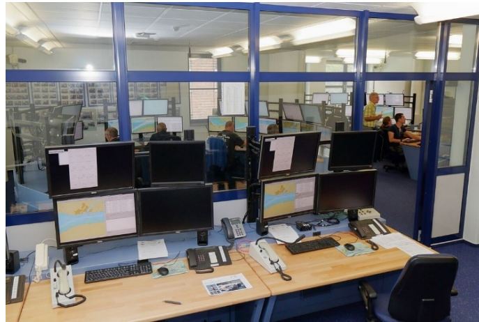
Figure 1: Instructor area of VTS-Simulator in the Maritime Simulation Centre Warnemünde (MSCW) – separate room with communication means, 5 monitors to follow and control the scenario.
