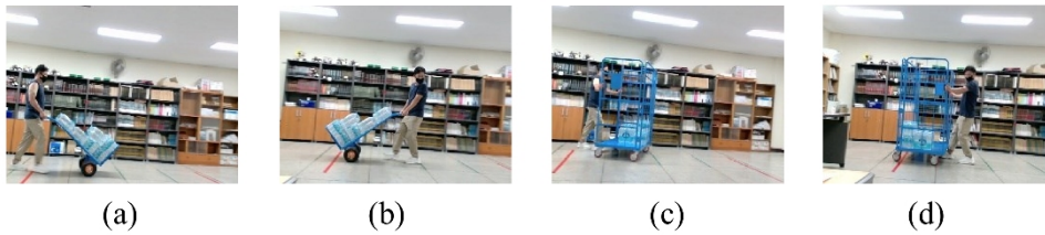
Figure 3: Experimental tasks: (a) hand cart pushing, (b) hand cart pulling, (c) rolltainer pushing, (d) rolltainer pulling.
