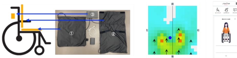
Figure 1: The seating assist device (left: appearance, middle: heatmap, right: icon).
