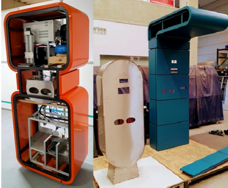
Figure 7: Basic variants of device housing.
