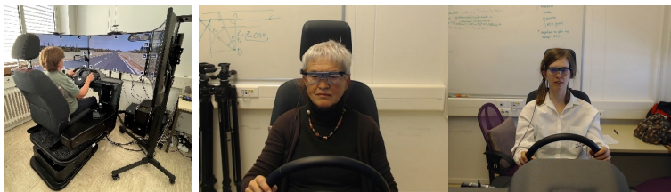
Figure 1: Driving simulator set-up and participants in the study equipped with Tobii 2 Glasses eye tracker.
