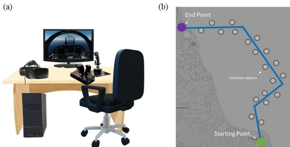
**Figure 1:** (a) Experimental set-up, including a HOTAS system and Head-Mounted Display (HMD), (b) Flight route with the position of unknown objects.
