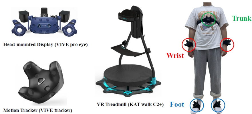
Figure 2: VR devices and location of tracker attachment.
