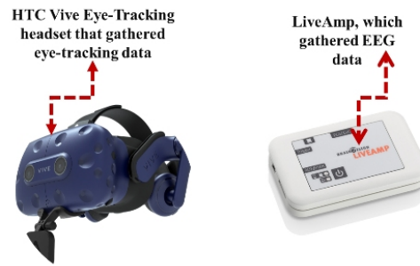
Figure 4: EEG amplifier and eye-tracking headset setup.
