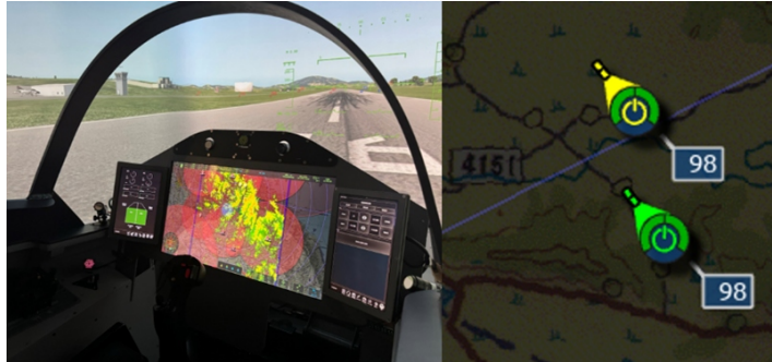
Figure 10: MUM-T Jet Simulator with UAV symbols on the tactical map.
