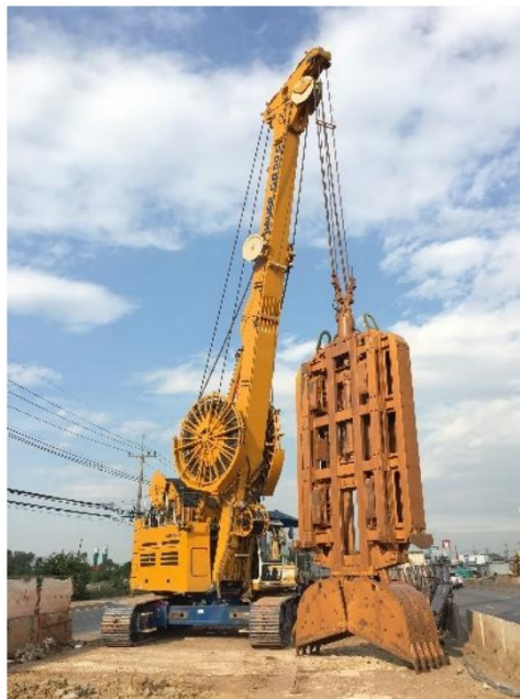
Figure 1: Exemplary construction equipment: hydraulic grab carrier (BAUER Maschinen GmbH).
