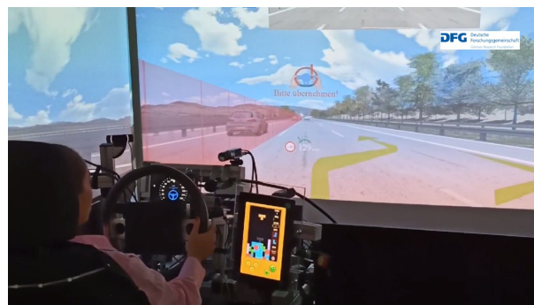
Figure 2: Driving simulator study setup. One of three groups of participants received extensive HUD feedback (design 3; red “wall” and green arrow as displayed in the figure).
