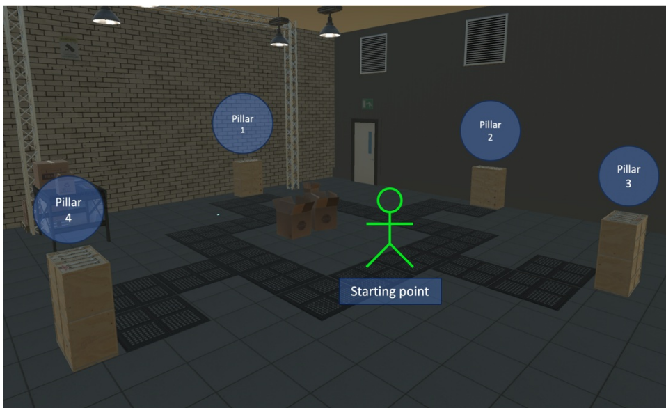
Figure 3: The VR warehouse scenario in which the test subjects had to navigate to and select the highlighted object on one of the four pillars. Leaving the grid-marked path triggered the warning effects.
