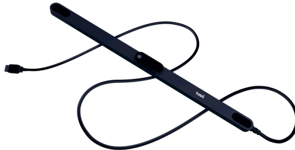
Figure 2: Figure of the Tobii 5 eye tracker hardware that was used in the experiment.
