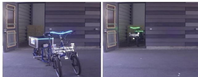
Figure 1: E-cargo bike with the visual communication concept in the begin parking process scenario with turquoise LED band (left) and end parking process with green signal (right).
