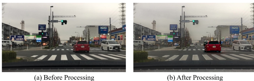
Figure 4: Gaze guidance processing results combining resolution control and color control. In (b), the red car appears more vividly red. Conversely, the saturation and resolution of regions outside the guidance target is diminished.
