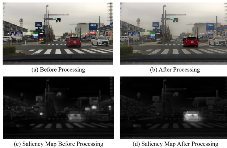
Figure 3: Gaze guidance processing results with color control. In (b), the red car appears more vividly red. Conversely, the saturation of regions outside the guidance target is diminished.
