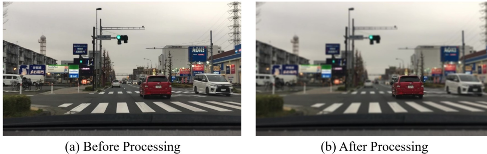
Figure 1: Gaze guidance processing results with resolution control. The red car in (b) is depicted with high resolution while the surrounding area is shown with reduced resolution.
