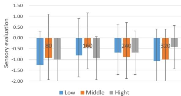
**Figure 5:** Sensory evaluation of seating comfort based on differences in tire air pressure.
