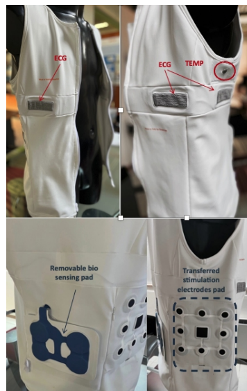
Figure 4: Sensors integrated in the inner side of the GAMMA garment.
