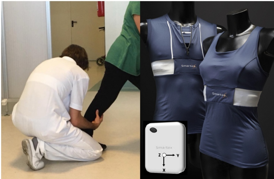
Figure 1: On the left, the physiotherapist during a monitoring session, on the right male and female models of WWS with the RUSA device (not to scale) with reference axes.
