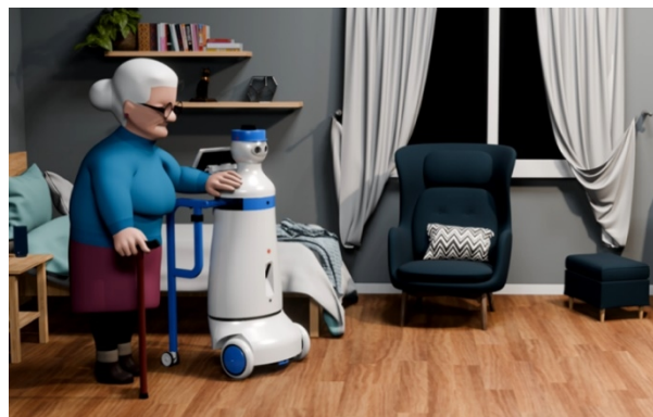
Figure 3: Special risk case: a person is leaning to the robot when it starts moving.
