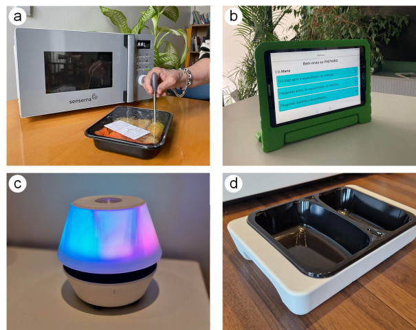
Figure 2: PREPARIO system components: a) the microwave oven with the wireless temperature probe, b) the survey app for end-users, c) the smart home voice assistant EMMA, d) the food tray with built in sensors.
