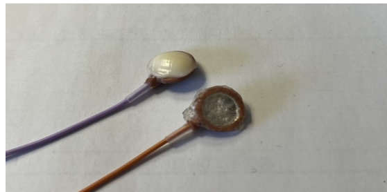
Figure 1: A purple cable electrode coated with conductive paste and an orange cable electrode coated with a transparent conductive gel sheet.
