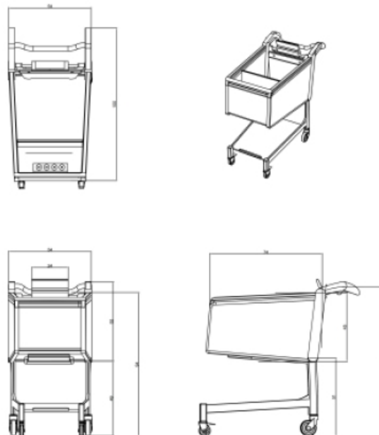
Figure 2: Three views and dimensions of improvement design of age-friendly supermarket shopping carts based on Ergonomics.
