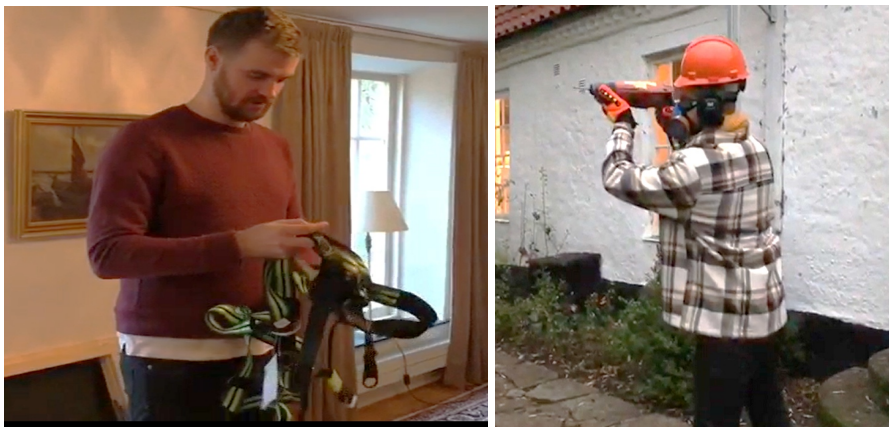
Figure 1: Snapshots from usability test videos, featuring a guessability test of a safety harness (left), and a demonstration of simultaneous use of PPE - including helmets, hearing protection, protective glasses, respiratory protective equipment, gloves - along with a drill, over a specified duration (right).
