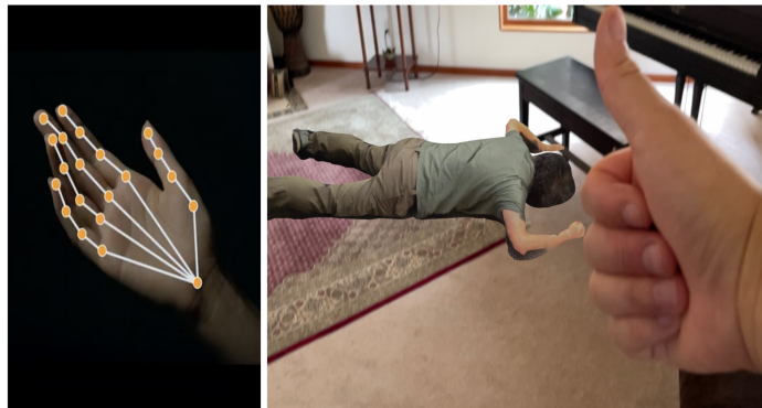
Figure 8: Hand tracking using Apple Vision kit to control the avatar face up or down.
