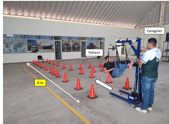
Figure 6: Course A layout. Course has a linear distance of 8 meters. Front wheel was aligned to start line.
