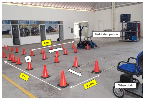
Figure 7: Course B layout. Course had a length of 8 meters by 93 centimeters wide. Course had a 90° turn [to left (A)]. Were used traffic signs (located 1 meter separated between them) in order to limit the course. Rear Wheel was aligned to start line of course.
