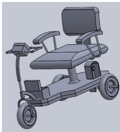
Figure 1: Isometric design of the electric wheelchair (source: own).
