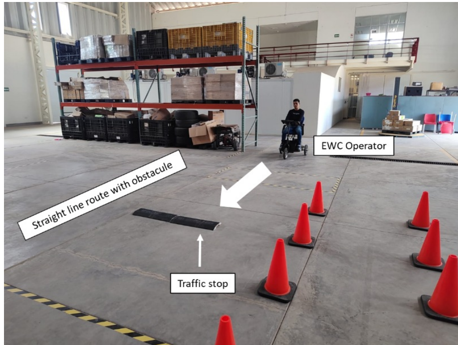
Figure 8: Course C layout. Course had a length in line of 15 meters, with an obstacle (traffic stop) at the middle. Front wheel was aligned to start line.
