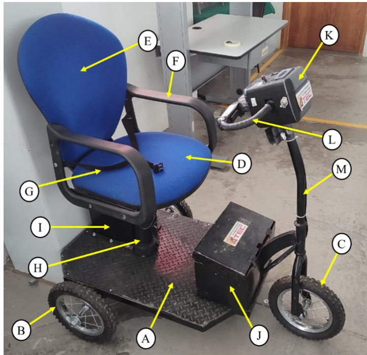
Figure 5: Electric wheelchair completed (source: own). (A) Chassis, (B) rear anti-tip rim, (C) front anti-tip rim, (D) seat, (E) backrest, (F) armrest, (G) seat belt, (H) seat base mast, (I) traction system box, (J) power supply box, (K) control box, (L) steering wheel, (M) steering wheel mast.
