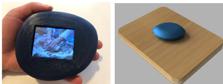
Figure 5: a) The Pebble interactive device; b) a Pebble and the base station tray.
