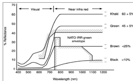
**Figure 3:** Four-color spectral reflectance curves.
