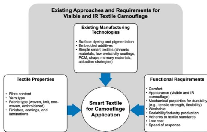
**Figure 2:** Camouflage technologies for smart textiles.
