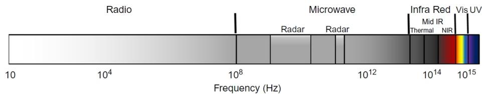
**Figure 1:** The electromagnetic spectrum from radio waves to UV light.
