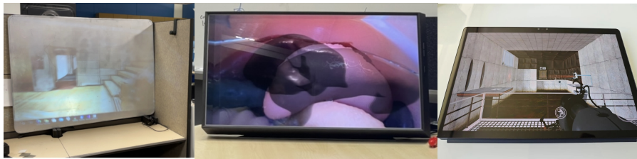
Figure 2: Open stereo displays (stereo projector, Looking Glass, and Lume Pad 2).
