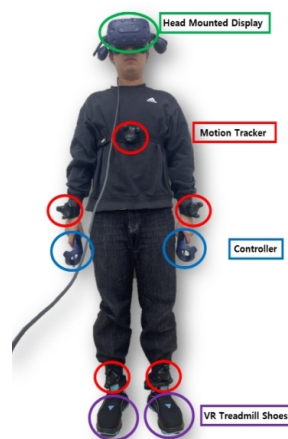
Figure 4: Location of tracker attachment.
