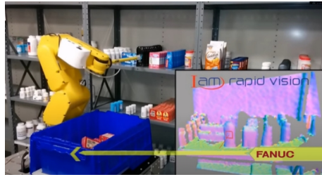
Figure 5: Shelf picking with vacuum suction cup ( Robotic Shelf Picking - IAM Robotics Automated Storage & Retrieval System (AS/RS) - YouTube, 2015 ).
