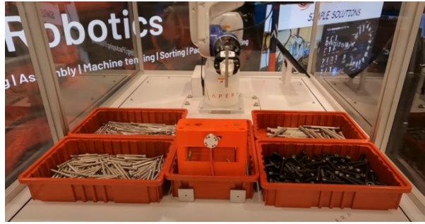
Figure 3: Screw bin picking system ( bin picking, kitting and sorting of bolts with an Epson industrial robot—multiple object finishes - YouTube, 2023 ).
