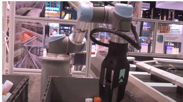
Figure 2: Bin picking system in e-commerce. ( Bin-picking and packaging - powered by robots - enabling e-commerce growth - YouTube, 2017 ).
