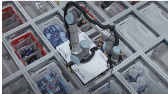
Figure 1: Ocado on-grid bin picking system. ( Introducing On-Grid Robotic Pick - YouTube, 2022 ).
