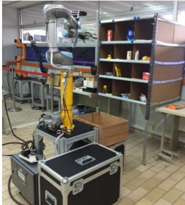
Figure 10: Strategy based shelf picking system (Zhu et al. , 2016).
