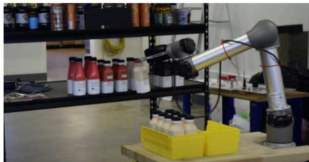
Figure 4: Shelf picking with two-finger grippers ( Robotic Materials Inc.’ GPR-1 in a shelf restocking task - YouTube, 2019 ).
